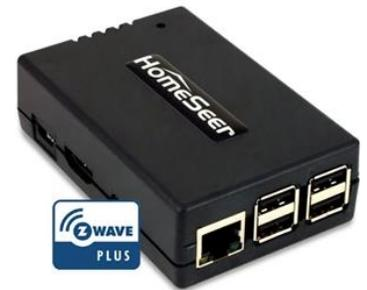
Battery operated devices should be right next to the Z-Wave controller when adding. Door Locks should be no more than 10 feet away when being added and should be removed first.
